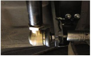
15. By screwing the ball joint into the rod attach the bush end of the rod to the axle bracket, do not tighten just yet. The rod length should be neutral and not required to be pulled or pushed to engage the Axle Bracket/Bush bolt cleanly. (See Image below)
