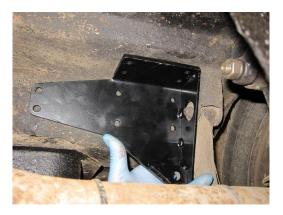
6. Pilot drill the holes, re-drill to 8mm and then pass the bolts with large washers through the boot floor and secure the bracket using the plain nuts. (See Images below)
