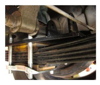
13. Assemble and evenly tighten the U bolt nuts. (There is no torque specified in the workshop manual for these but we'd suggest 25 to 30 ft/lbs)
